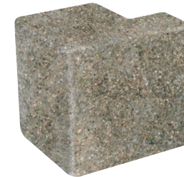
6620 SQUARE CONCRETE STEP Matching square concrete step for square concrete pedestals. Steel-reinforced, pre-cast construction with air-entrained concrete to ensure 5000+ PSI compressive strength with exposed aggregate finish. 10" (25.4 cm) high for surface mounting.
